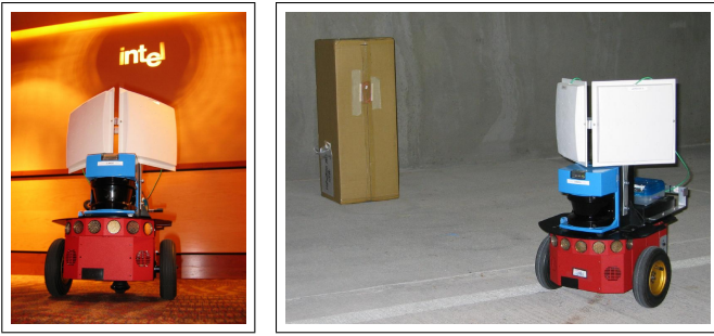
Fig. 2. Pioneer 2 with Sick Laser Range Finder, RFID reader and two antennas (left). Experimental setup used for learning the likelihood function of tag detections (right).
