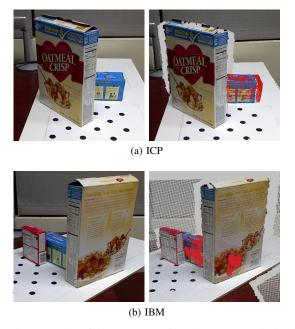
Fig. 5: Example failure cases for the two optimization techniques; original scene on the left, pose optimum on the right, with the Ziploc box model overlaid in red. In ICP (top), free-space protrusions occur because free-space information is not used. IBM failures (bottom) can occur when occlusion is present blocking all edges along one direction.
