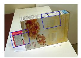
Fig. 1: Scene with clutter and occlusion. Matching the small box based on its 3D model is problematic. ICP will match the model with free-space protrusions, as on the occluded box at left. The beam model will find the correct match there, but will prefer to embed the smaller box model into the larger box, where the whole front surface matches.
