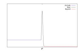
Fig. 2: Piecewise sensor model used in IBM. On the x-axis is the beam measurement  $d_i$ .  $d_i^*$  is the expected measurement from the model. Not to scale.
