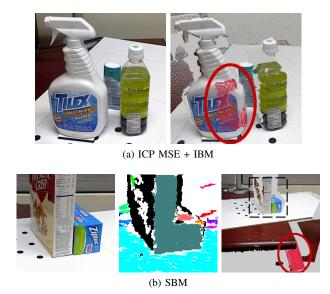
Fig. 6: Example failure cases for the restart evaluation functions. (a) ICP MSE and IBM sometimes select matches to similarly shaped, though differently sized objects, as with this toothpaste bottle. (b) Under-segmentation in SBM leads to a lack of surfaces against which to match. Here the Ziploc bags and cereal box are segmented as the same object.
