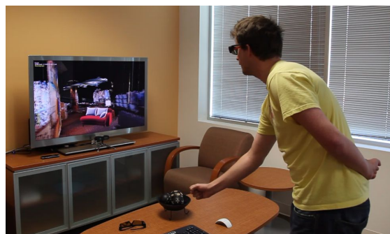
Figure 11. A gesture-controlled flythrough system running on a 3D TV. The user uses hand gestures to navigate through a virtual space being rendered in real-time; he can also use gestures to place a downloaded sofa model into the constructed model.
